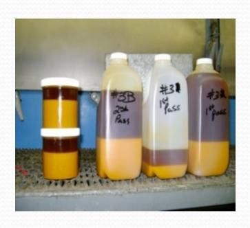
As you can see in the picture to the left, when you run the biomass through expellers and presses at the correct temperatures and pressures, they have the ability to effectively remove oil from the oil rich biomass
