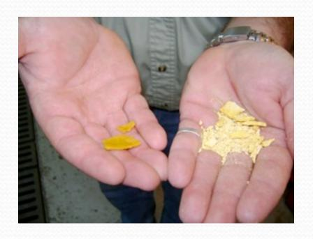
In the picture to the left, you will notice the difference between an algae biomass that has been fully extracted using a press and the white product with less residual oil is after solvent extracting the product
