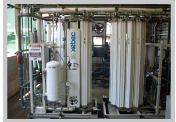
XEBEC's compact and reliable M-3200 gas purification system proved a perfect fit for Scenic View Dairy.
