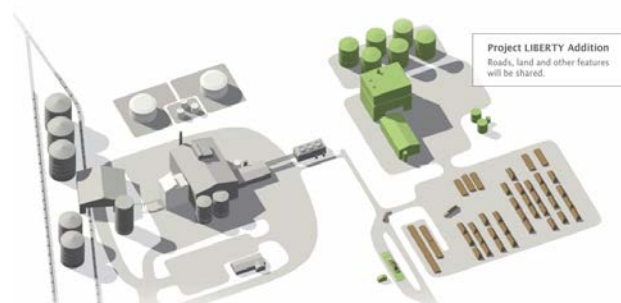
Fig. 2. Bolt-on facility under construction by POET-DSM in Emmetsburg, IA. Conventional corn ethanol plant on left and cellulosic stover plant on right.
