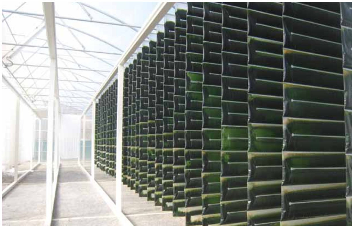
Figure 9: Valcent’s High Density Vertical Growth (HDVG) systems grow algae with only light, water, and air in a closed loop, vertical system of polyethylene sleeves in greenhouses.
