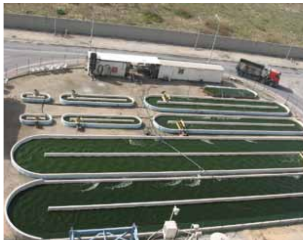
Figure 5: Open raceway ponds with paddle wheels (far right) for circulating the water.
