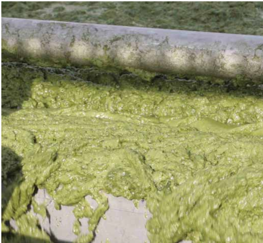
Figure 16: Algae and phosphorous after undergoing dissolved froth flotation. Phosphorus from the effluent of wastewater treatment ponds can be removed by chemical precipitation of the soluble phosphorous and then the solids, formed together with the algae, are separated from the water by flotation.
